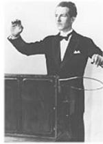
**1917:** Leon Termen invents the Theremin (*left*). Termen sought to free the performer from the keyboard and fixed intonation by making use of the influence of body capacitance on the heterodyning effect between two high frequency sound waves. Moving the right hand alters pitch, and the left changes the volume. The idea is of some interest to this project.
