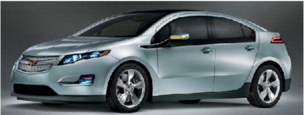
25 kWh per 100 km (running on electric power alone)
