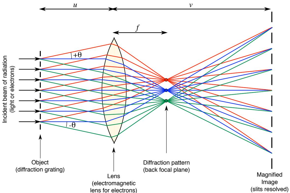
Fig. 1. Abbe theory of imaging using all diffracted spots
