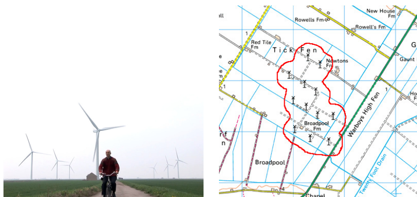
Figure 9. Red Tile wind farm, East Anglia, and its associated land area. The blue grid's spacing is 1 km. Each turbine has a diameter of 82 m and a capacity of 2 MW. Map © Crown copyright; Ordnance Survey.
