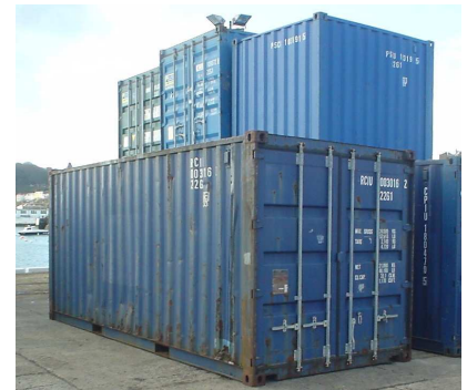
Figure I.4. A twenty-foot container (1 TEU).
