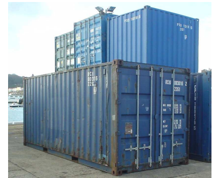
Figure I.4. A twenty-foot container (1 TEU).
