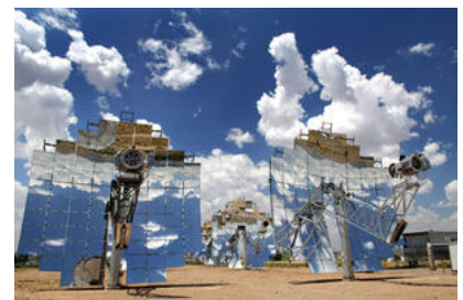
Figure 1.2. Stirling dish engine. These beautiful concentrators deliver a power per unit land area of 14 W/m 2 . Photo courtesy of Stirling Energy Systems. www.stirlingenergy.com
