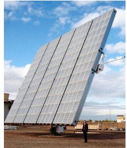
Figure 1.1. A 25 kW (peak) concentrator photovoltaic collector produced by Californian company Amonix. Its 225 m 2 aperture contains 5760 Fresnel lenses with optical concentration \times 260 , each of which illuminates a 25%-efficient silicon cell. One such collector, in an appropriate desert location, generates 138 kWh per day – enough to cover the energy consumption of half an American. Note the human providing a scale. Photo by David Faiman.
